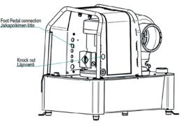
The foot pedal enables holding the hose assembly with both hands. In P32NMS and P20NMS machines foot pedal is **double pedal**.
