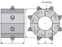
With standard dies. Crimping range can be increased with special dies.
